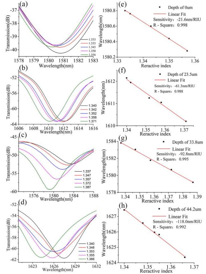
Fig. 5. (a)-(d) transmission spectra response versus RI for the SPCO fiber MZI structure with different polished depths of 0, 23.5, 33.8 and 44.2  $\mu\text{m}$ , respectively; (e)-(h) Dip wavelength shift as a function of RI.
