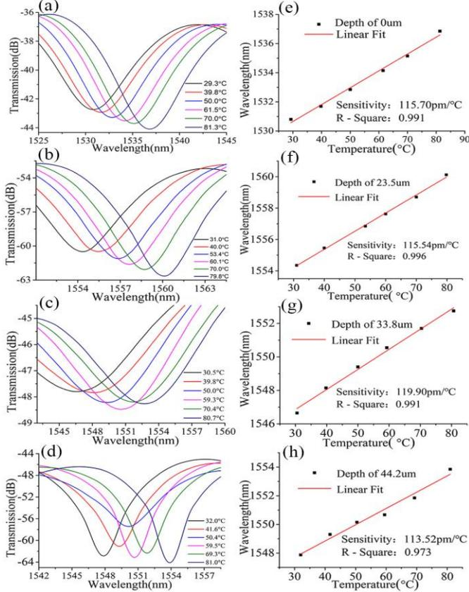
Fig. 6 (a)-(d) transmission spectra response versus temperature for the SPCO fiber MZI structure with different polished depths of 0, 23.5, 33.8 and 44.2  $\mu\text{m}$ , respectively; (e)-(h) Dip wavelength shift as a function of temperature.
