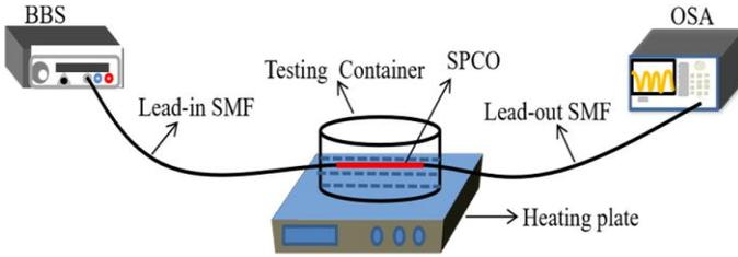
Fig. 4. Structural device for RI and temperature measurement.
