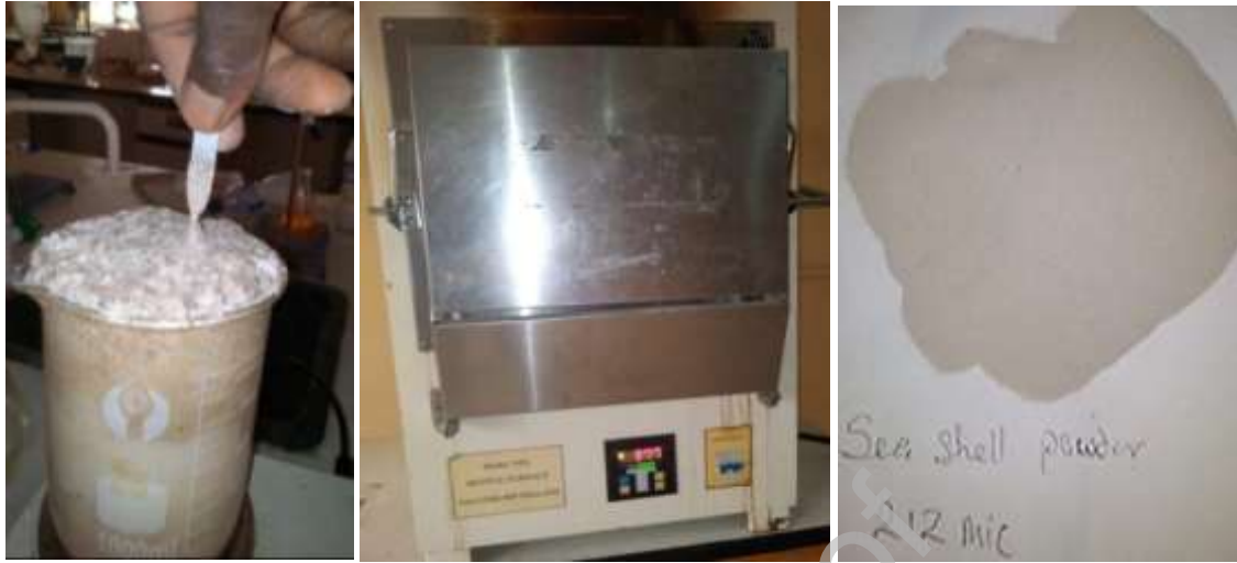
Fig. 2. Model SXL maple furnace for preparation of African land giant and sea snail shell
