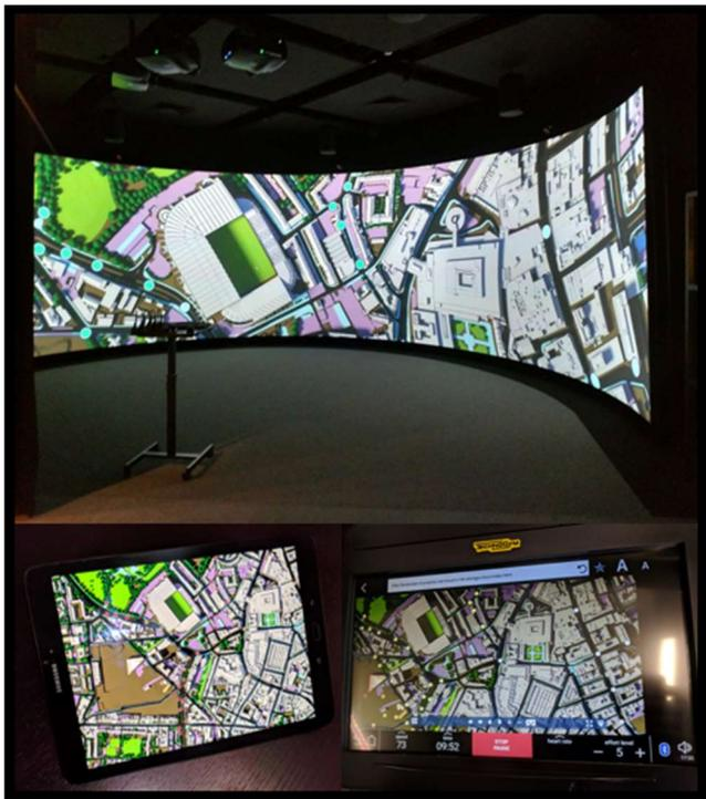
Fig. 9. The hierarchical krpano image format for serving the visualization to users from Azure Blob store allows it to be viewed interactively on a wide range of thin client devices, shown here anti-clockwise from top are the 8 Mpixel Curtin HIVE cylinder, a Samsung Galaxy S3 and on our local gym cycling machine.
