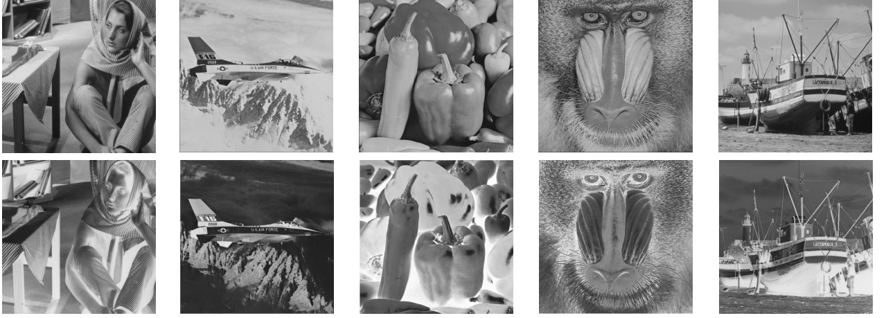
Figure 8: Visual difference between the images decrypted with the correct key and those decrypted with its flipped version. First row: decryption using the correct key. Second row: decryption using the flipped version of the correct key.
