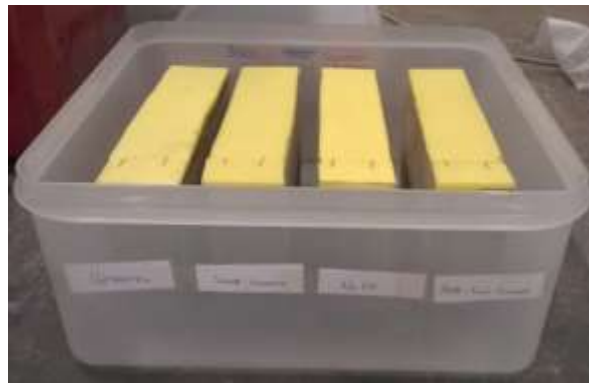
8 9 Figure 9. Set- up of contact test
