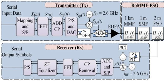
Fig. 2: Theoretical model of RoMMF-FSO system
