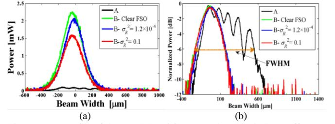
Fig. 5: Beam profile of the RoMMF-FSO system shown turbulence effect on: (a) Amplitude, and (b) FWHM
