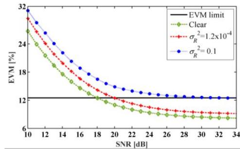
Fig. 10: Analysed EVM performance for FSO span of 500 m
