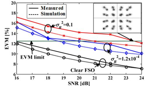
Fig. 9: Measured and theoretical EVM performance of the setup C under clear air condition and two weak turbulence levels
