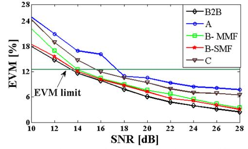
Fig. 7: Measured EVM performance of the RoMMF-FSO system
