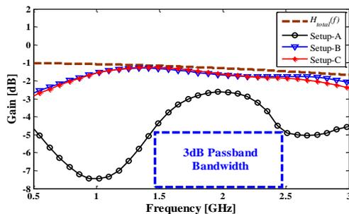
Fig. 4: Transfer function of the RoMMF-FSO system
