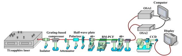
Fig. 2. Schematic of the experimental set-up used.
