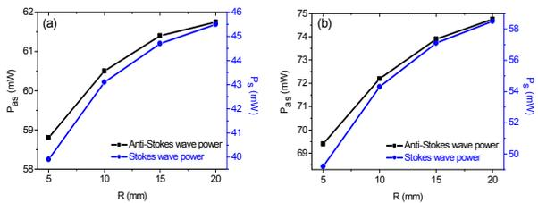
Fig. 5. The dependence of anti-Stokes wave power  $P_{as}$  and Stokes wave power  $P_s$  on the fiber bending radius  $R$  for pump pulses injected along the (a) slow and (b) fast axis, respectively. The pump wavelength  $\lambda_p = 800$  nm and average input power  $P_{av} = 500$  mW.
