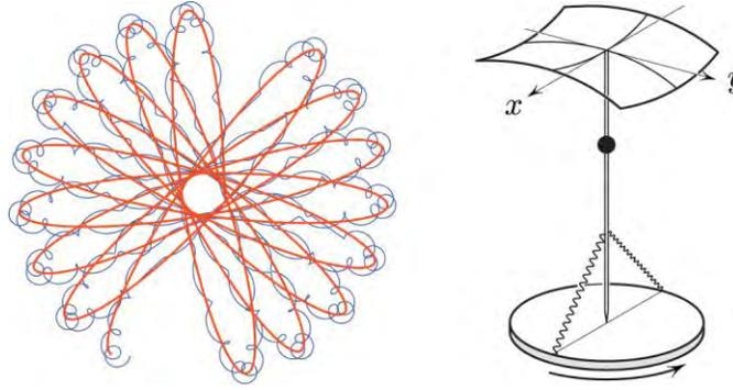
Fig. 2 (Left) Trajectory of the guiding center  $u$  (thick curve) tracking the corresponding trajectory  $x$  (thin curve). The view is in the inertial frame with  $\varepsilon = 0.45$ . (Right) A possible mechanical realization of the rotating saddle trap. Here,  $x$  and  $y$  are the angular variables of the inverted pendulum, and the graph of the potential energy is shown (figure adapted from [12]).
