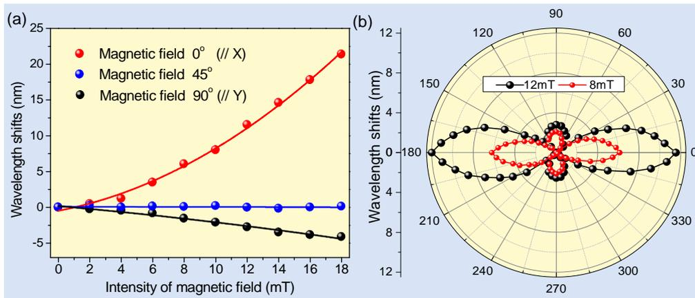
FIG. 4. (a) Wavelength shift of the TFBG-SPR to magnetic field intensity for three different orientations; (b) Absolute value of the wavelength shift to magnetic field orientation (with TFBG tilt plane at  $90^\circ$ ), for two values of magnetic field intensity. (Multimedia view 2)
