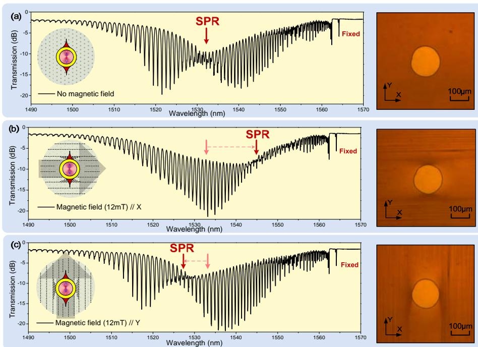
FIG. 3. Left: Plasmonic TFBG spectral responses, (a) without magnetic field, (b) with magnetic field along the horizontal (X) direction, (c) with magnetic field in the vertical (Y) direction. Right: microscope image of the magnetic fluid clusters formed around an air bubble (with diameter close to a standard SMF). (Multimedia view 1)
