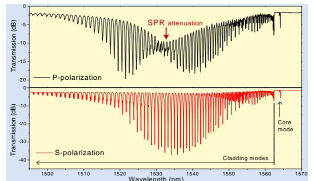
FIG. 2. Transmission spectra of TFBG coated with 50 nm of gold and immersed in magnetic fluid, for P-polarized incident light (top) and S-polarized incident light (bottom). The SPR location corresponds to the spectral notch near 1530 nm in the upper graph.
