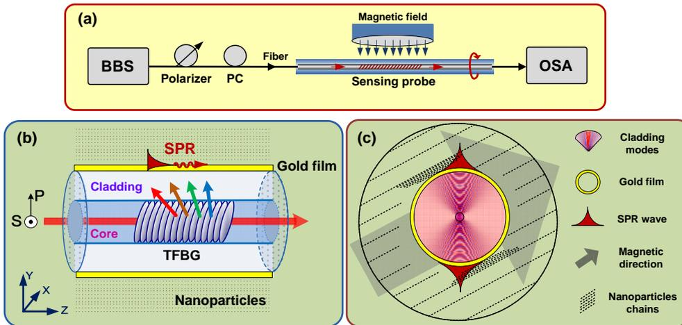
FIG. 1. (a) Schematic diagram of magnetic sensing system; (b) polarimetric TFBG with linearly polarized light emitting for SPR excitations; (c) cross section of TFBG and ferro-nanoparticles sealed in a capillary tube under an external magnetic field.
