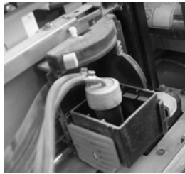
Figure 1: Z-Corps 3D Printer, Printer Head Cap
