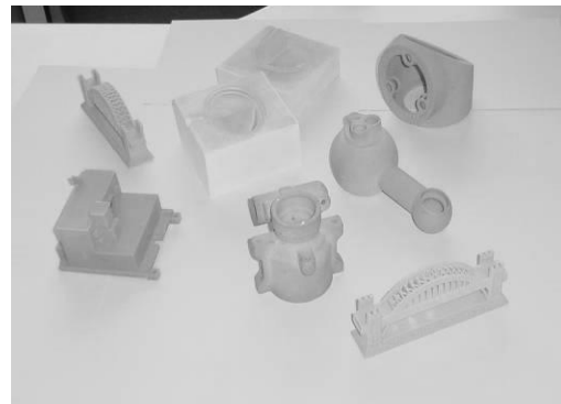
Figure 7: Parts Manufactured on LOM machine in the CRPD Figure 8 : Parts Manufactured on Z Corps 3D Printing Machine
