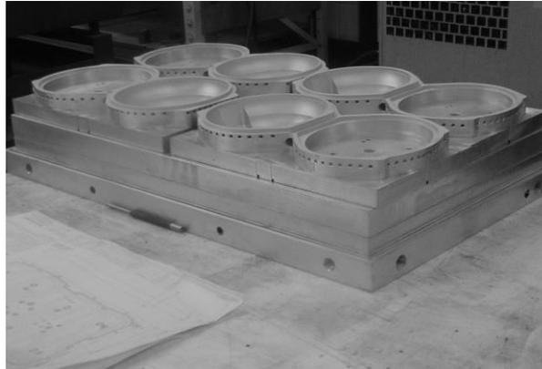
Figure 4: Multi – Cavity Mould Tool
