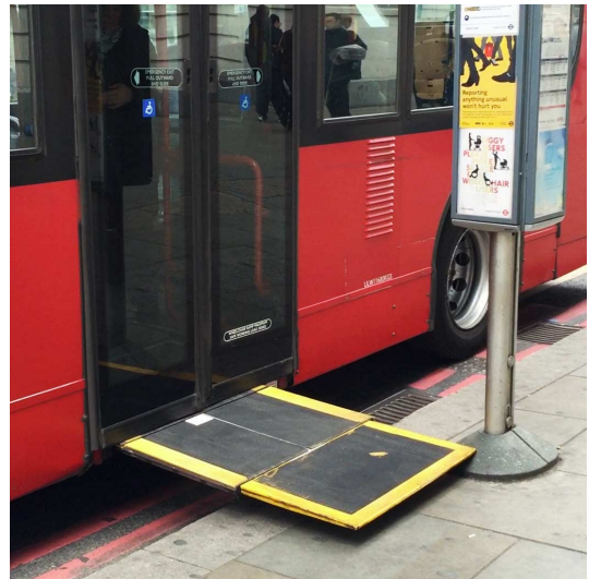
Figure 2: A bus ramp obstructed by street furniture, which would not support the weight of a powered wheelchair. After able-bodied passengers disembarked, the bus moved forward and redeployed the ramp before our participant could get off.
