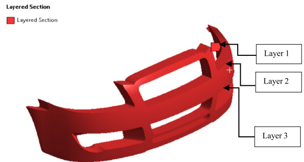
Fig. 6 The layered orientation of bumper made using jute material
