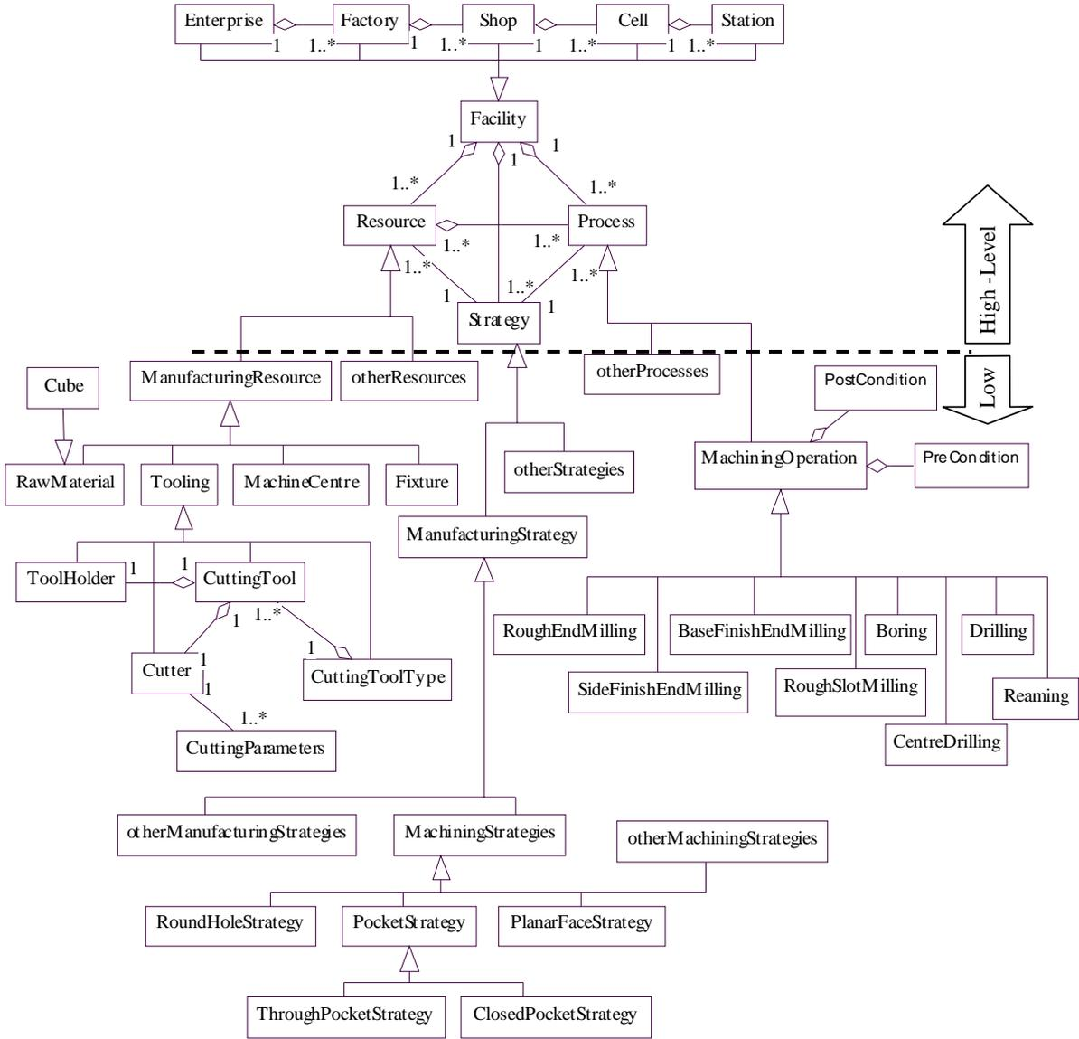
**Figure 6 Manufacturing data model in UML representation**
