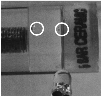
c) Bubbles that emerged from ceramics and crevice t = 22.5 ms or t_{log} = 13.7610 s suction \approx 100 kPa.
