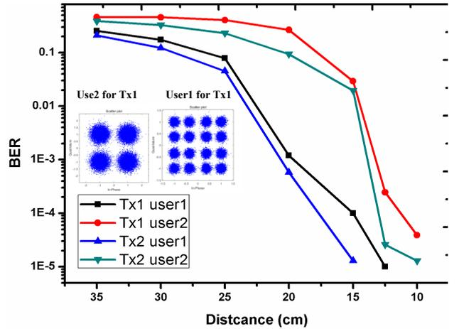
Fig. 3. BER performance with 4-QAM mapping for user 1 & 2.
