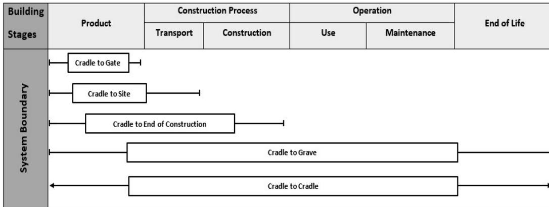
Figure 2: System Boundaries of EC Estimation
