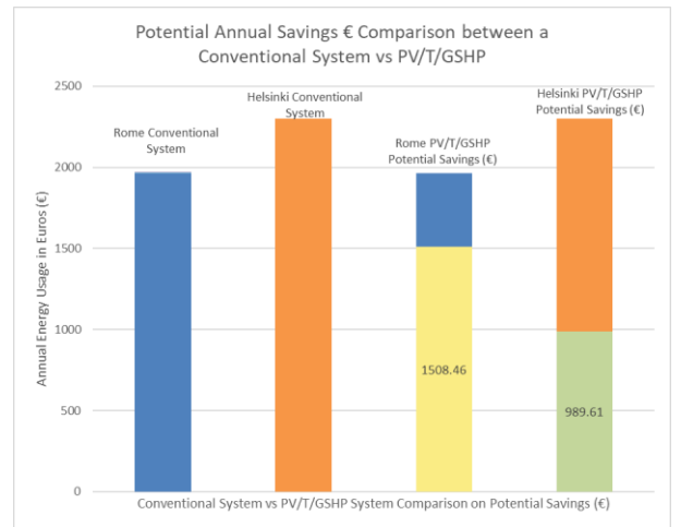
Fig. 6: Potential Annual Savings € Comparison between a Conventional System vs. PV/T/GSHP
