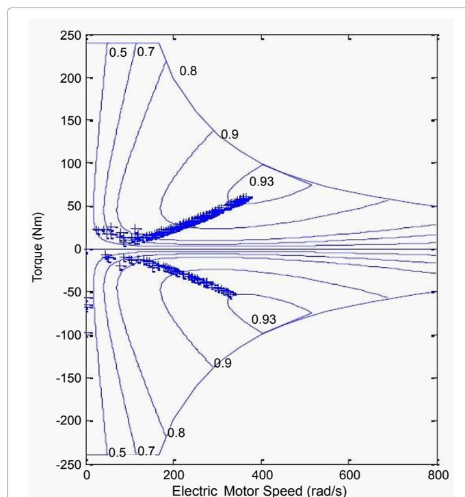
Figure 12: Motor operation points with continuously variable gear.
