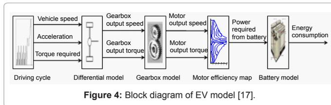
Figure 4: Block diagram of EV model [17].
