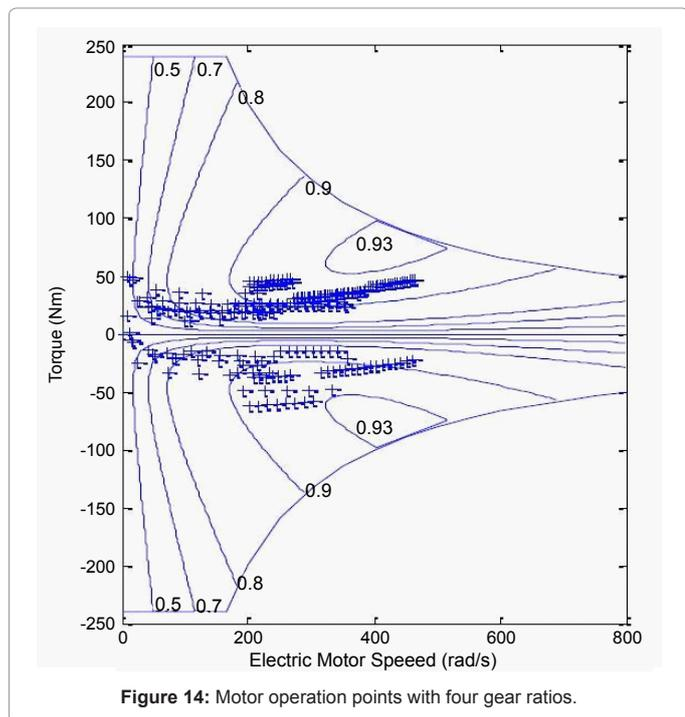
Figure 14: Motor operation points with four gear ratios.
