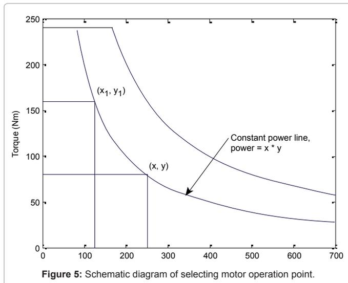
Figure 5: Schematic diagram of selecting motor operation point.
