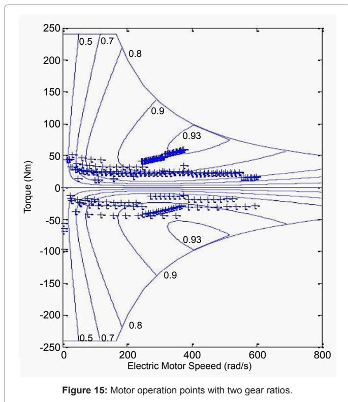
Figure 15: Motor operation points with two gear ratios.
