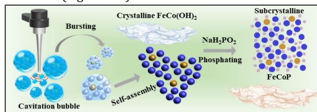
Figure 1 Schematic diagram for the fabrication processes of FeCoP ultrathin nanosheets.
