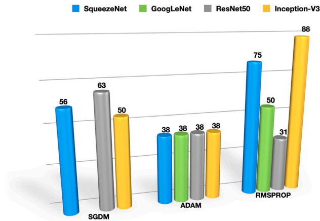
Fig. 7. Three class testing accuracies (%) tool wear classifications.
