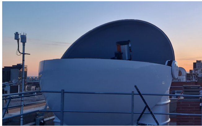
Fig. 3. Image of TURBO instruments on the roof of UPC. The all-sky camera and weather sensor are on the left, while TURBO1 is enclosed within the dome on the right.
