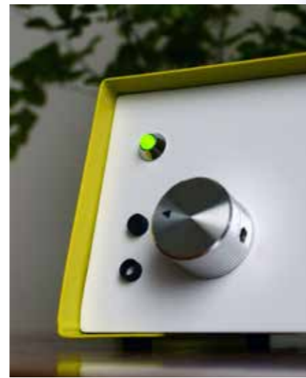
Figure 5. On-Off Swivel. Photo: Anne Spaa. 7½ can be set to the ‘on’ or ‘off’ state using a swivel switch. The rigid aluminium swivel with a switch mechanism requires a bit of force to rotate. This as, although 7½ only has one control, the interaction with it should feel significant; it starts the important period of sleep. When turned ‘on’, the swivel points at the solid circle.
