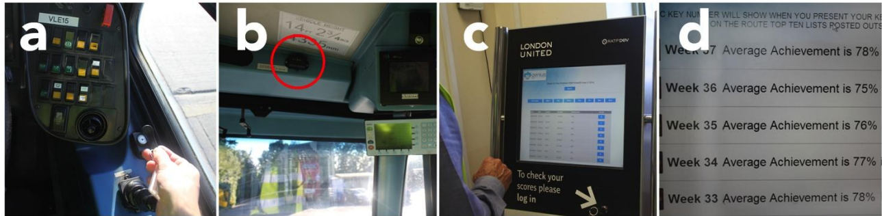
Figure 1. From left to right: a) Placing the Drivewell key fob onto the reader; b) The Drivewell indicator in the driver's cabin (circled red); c) The Drivewell computer terminal; and d) close-up of computer terminal screen showing Drivewell scores.
