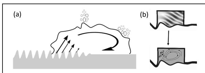
**Figure 1.** Schematic cross-sectional representation of the different fluidic actuations emerging from interactions between a SAW and a volume of liquid in a droplet (a), leading to deformations on the surface (and ultimately movement, jetting or nebulisation), as well as streaming and recirculatory flows, or within a microchannel (b).
