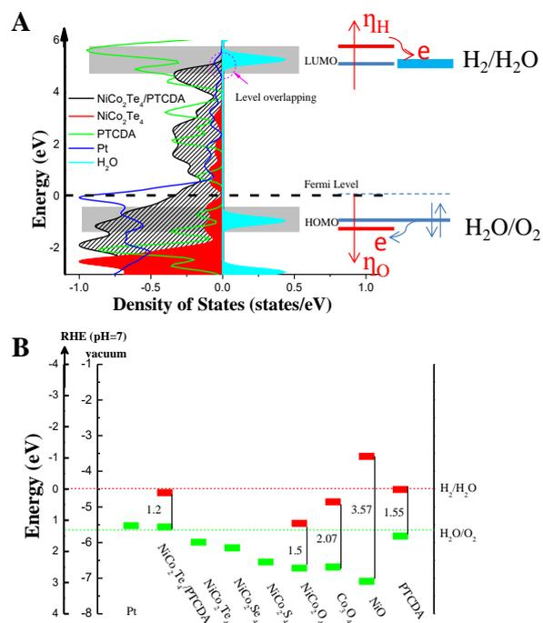
**Figure 5.** (A) The calculated density of states (DOS) of  $NiCo_2Te_4/PTCDA$  (black),  $NiCo_2Te_4$  (red), PTCDA (green), Pt (blue), and  $H_2O$  (cyan); (B) Bandgap energy, Valence band and Conduction band positions of several samples on an energy scale (eV) vs. RHE/Vacuum level.
