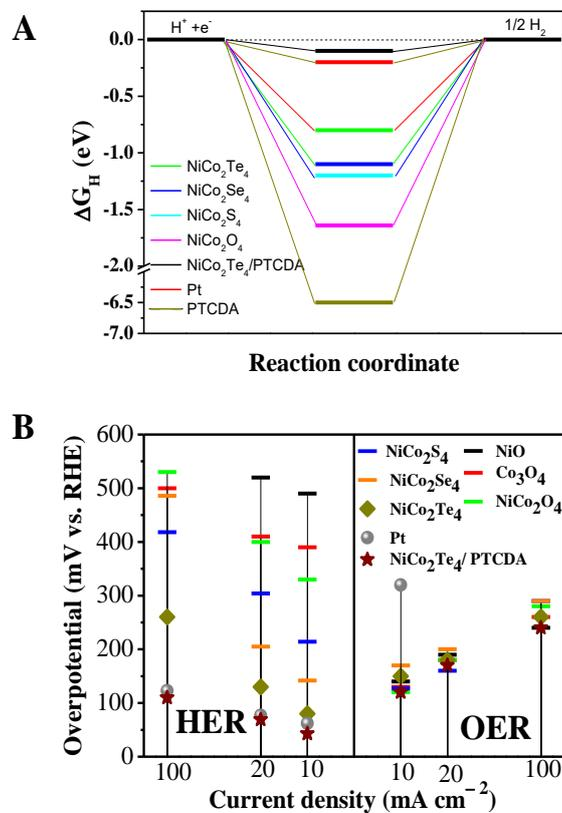
**Figure 6.** (A) Hydrogen adsorption free energy  $\Delta G_H$  diagrams; (B) Performance of catalysts (2 nm clusters of NiO,  $Co_3O_4$ ,  $NiCo_2O_4$ ,  $NiCo_2S_4$ ,  $NiCo_2Se_4$ ,  $NiCo_2Te_4$ ,  $NiCo_2Te_4/PTCDA$ , and Pt) for HER and OER. The overpotentials obtained at 10, 20, and 100  $mA\cdot cm^{-2}$  on various catalysts in 1 M PBS.
