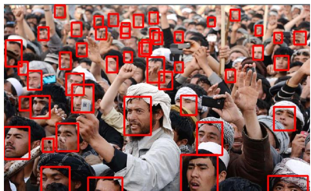
Figure 1: Example of deep neural network multi-resolution face detection, successfully identifying large and small faces.
