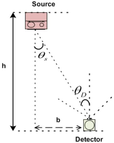
**Fig. 2: A VLC link with a Lambertian source**
