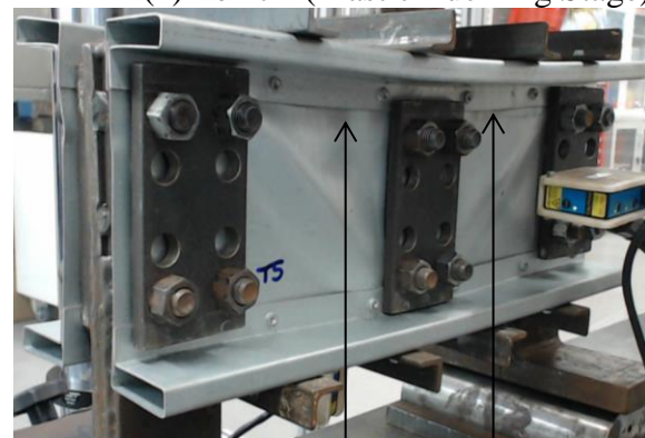
Small Separation in compression region
