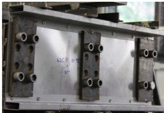
(c) 250x51x1.15x0.95 RHFCB (Test 7, AR of 1.0)
