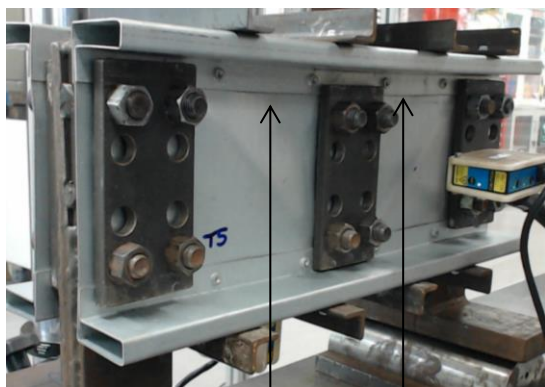
No Separation in compression region
