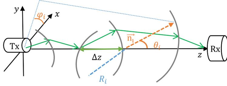
Figure 1. A schematic diagram of the system model consisting of the Tx, turbulent channel and the Rx
