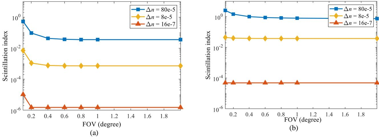
Figure 5. SI vs. the Rx's FOV for different values of  $\Delta n$  for: (a)  $L = 30$  m, and (b)  $L = 100$  m
