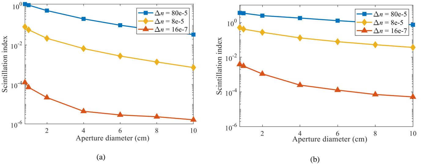
Figure 4. SI vs. the Rx's aperture diameter for different values of  $\Delta n$ : (a)  $L = 30$  m, and (b)  $L = 100$  m
