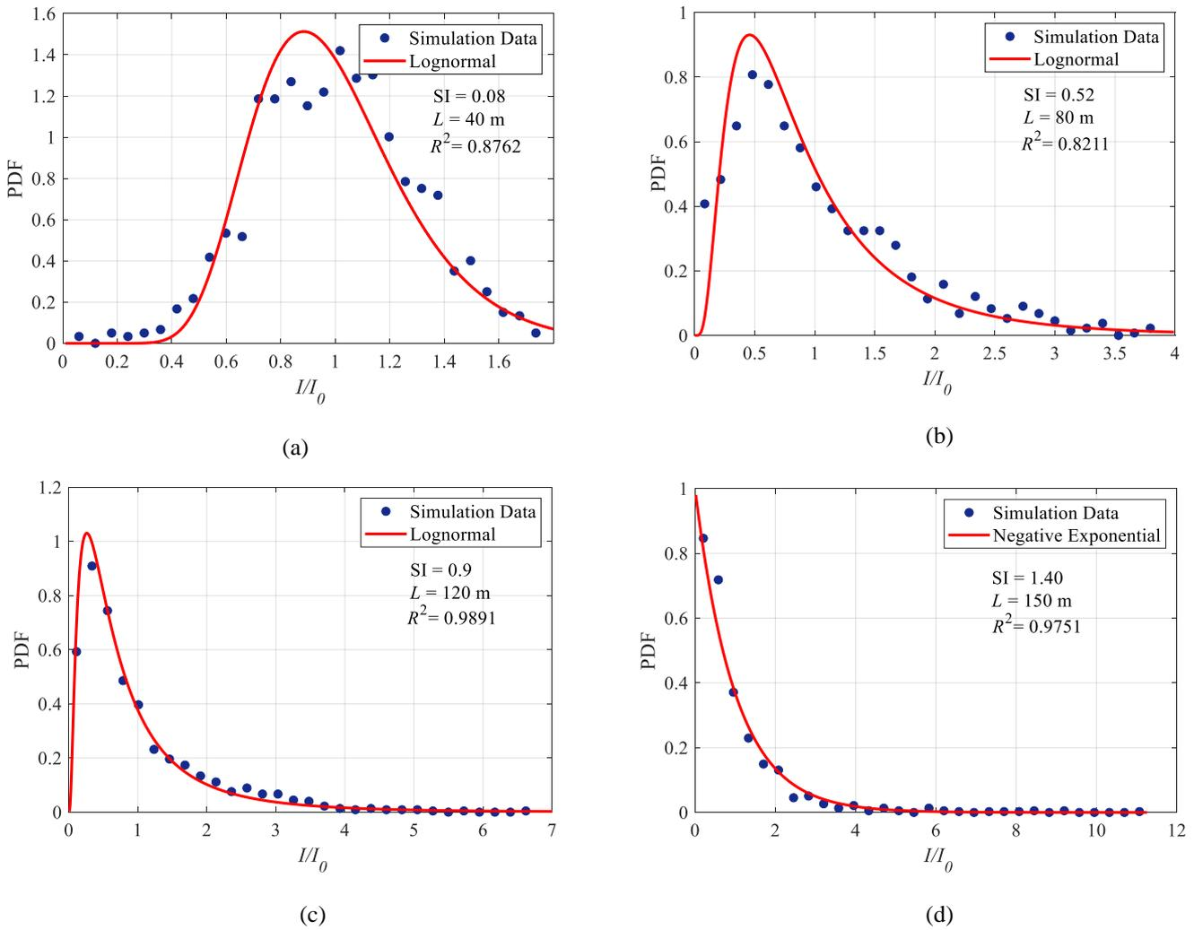
Figure 2. PDF of the simulated received light intensity vs. the normalized intensity fitted with lognormal and negative exponential distributions for: (a)  $L = 40$  m, (b)  $L = 80$  m, (c)  $L = 120$  m and (d)  $L = 150$  m
