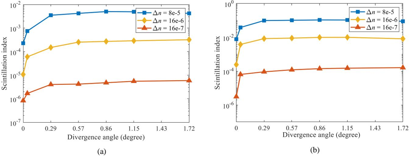
Figure 3. SI vs. the Tx's divergence angle for different values of  $\Delta n$ : (a)  $L = 30$  m, and (b)  $L = 100$  m
