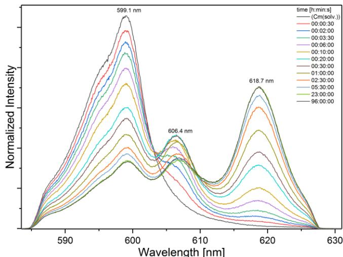
**Figure 8.** Normalized Cm(III) fluorescence spectra as a function of time after addition of ligand **10** in MeOH + 1.5 vol.% H<sub>2</sub>O ( $c(\text{H}^+) = 91.2 \text{ mM}$ ;  $c(\mathbf{10}) = 9.90 \times 10^{-8} \text{ M}$ ;  $c(\text{Cm(III)}) = 4.69 \times 10^{-8} \text{ M}$ ).
