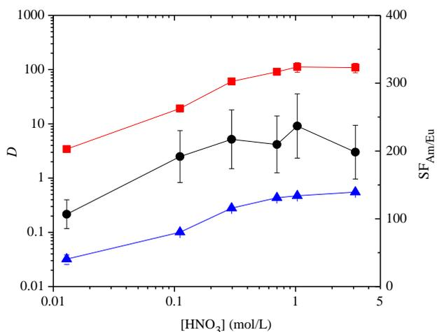
**Figure 2.** Extraction of Am(III) and Eu(III) by tetradentate ligand **10** in 1-octanol (0.01 M) as a function of the initial nitric acid concentration ( $D$  = distribution ratio, SF = separation factor, ■ =  $D_{Am}$ , ▲ =  $D_{Eu}$ , ● =  $SF_{Am/Eu}$ , mixing time: 60 min., temperature:  $22^\circ\text{C} \pm 1^\circ\text{C}$ ).
