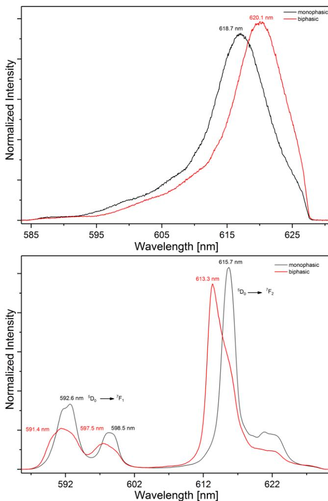
**Figure 11.** Comparison of the (black) fluorescence emission spectra of the  $[\text{M}(\mathbf{10})_2]^{3+}$  complexes in a monophasic batch experiment and (red) the formed complexes in the organic phase after extraction (Top:  $M = \text{Cm(III)}$ ; bottom:  $M = \text{Eu(III)}$ ;  $^5\text{D}_0 \rightarrow ^7\text{F}_n$  transitions ( $n = 1, 2$ )).
