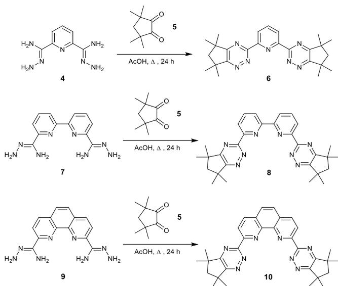
**Scheme 1.** Synthesis of bis-1,2,4-triazine ligands **6**, **8** and **10** containing 5-membered aliphatic rings from the  $\alpha$ -diketone **5**.
