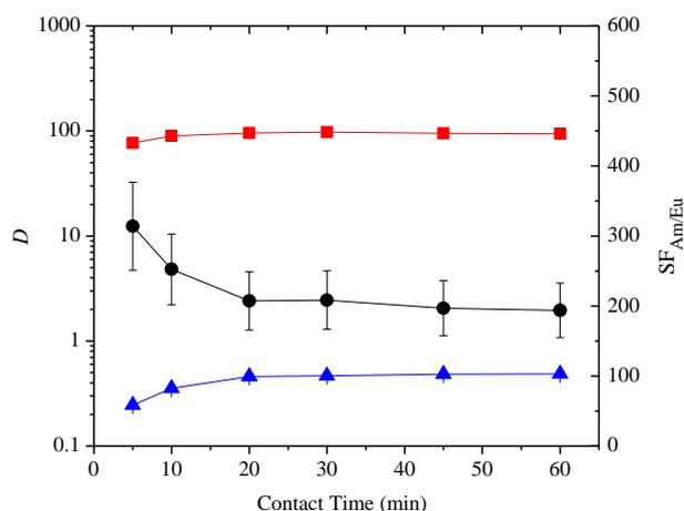
**Figure 3.** Extraction of Am(III) and Eu(III) from 1.03 M nitric acid by tetradentate ligand **10** (0.01 M) into 1-octanol as a function of contact time ( $D$  = distribution ratio, SF = separation factor, ■ =  $D_{Am}$ , ▲ =  $D_{Eu}$ , ● =  $SF_{Am/Eu}$ , temperature:  $22^\circ\text{C} \pm 1^\circ\text{C}$ ).
