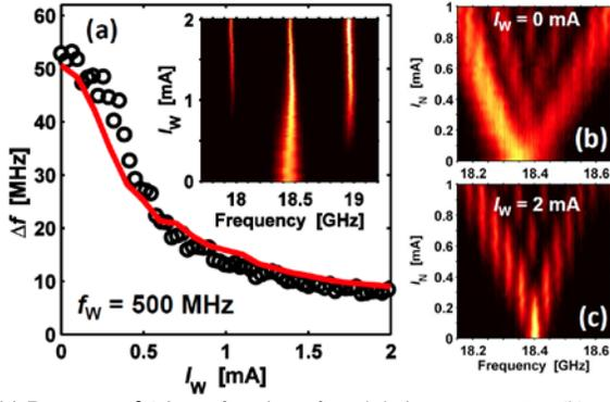
Fig 3. (a) Decrease of  $\Delta f$  as a function of modulation current,  $I_w$ . (b) and (c) highlight a double modulation experiment with  $f_N=40$  MHz and  $f_w=500$  MHz with modulation currents of  $I_w=0$  mA and 2 mA, respectively.
