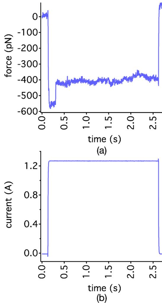
Fig.4 *A typical force trace captured while the feedback controller is tuned off, (a) an event happens at 0.306 s with an unbinding force of 102 pN. (b) the actuation current of 1.3 A starts at 0.133 s then is switched off at 2.621 s.*
