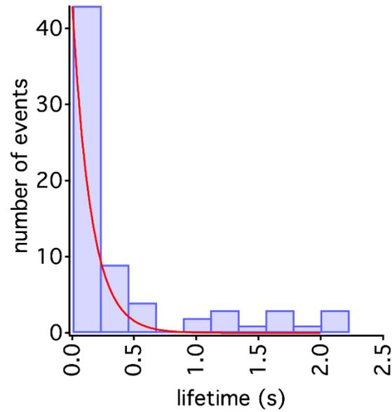
Fig.5. Histogram of lifetimes measured with a clamping force ranging from 40 pN to 55 pN. The mean value of the force is estimated as 47 pN corresponding to an expected lifetime of 0.394 s.
