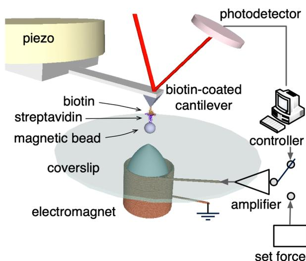
Fig.8. Schematic overview of the AFM setup. The input of the electromagnet is either controlled using the software-based controller during feedback ON case or it is driven with a constant set force input during feedback OFF case.
