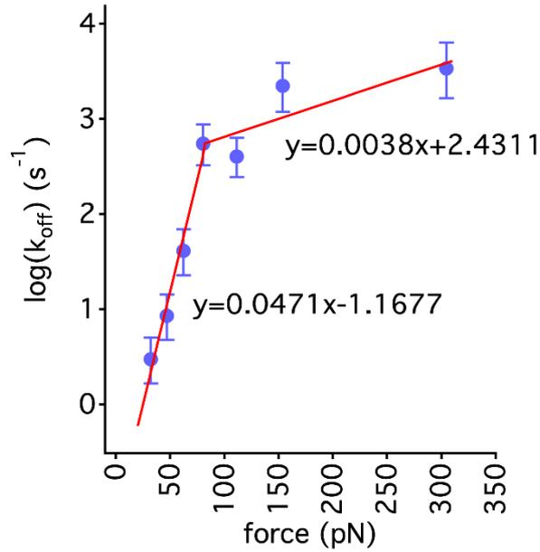
Fig.6 The variation of off-rate as a function of clamping force when the feedback controller is turned off.
