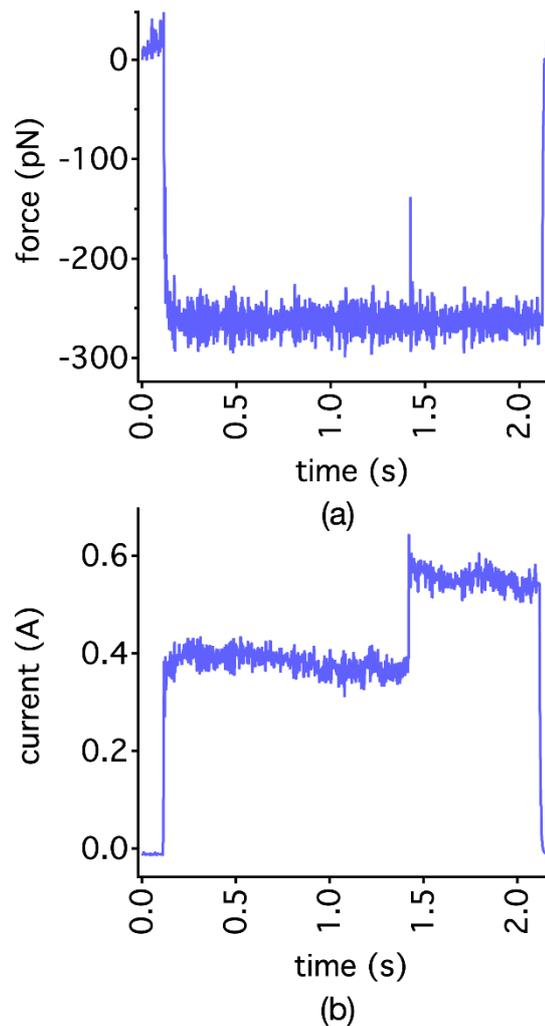
Fig.1 *A typical force trace captured when an event happens while the feedback controller is active at 1.419 s with an unbinding force of 120 pN, resulting in a jump in current by about 0.2 A.*
