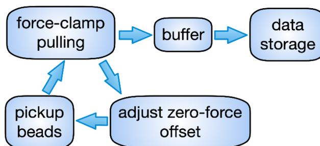
Fig.9. Block diagram of the software controller.
