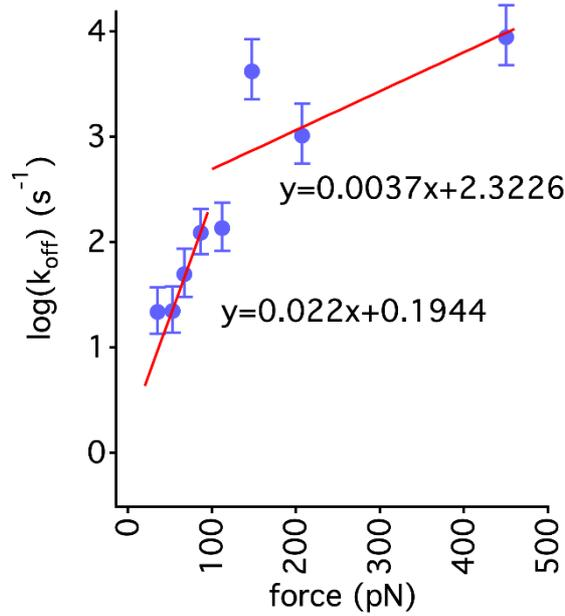
Fig.3 The variation of off-rate as a function of clamping force when the feedback controller is activated. The presence of two distinct energy barriers is obvious.
