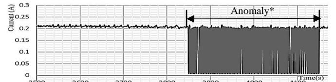
\*Malfunction in the cooling mode causing it to repetitively turn on and off
