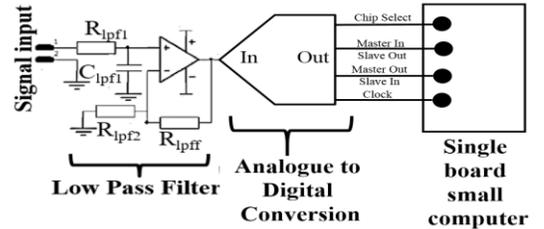
Fig. 4. Hardware system diagram of the slave meter
