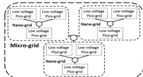
Fig. 1. ELV dc pico-grids forming into a micro-grid
