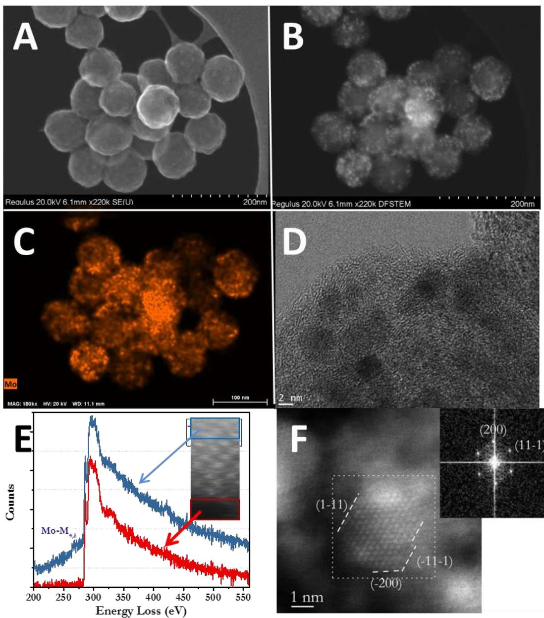
**Figure 2.** (A) Secondary electron (SE) SEM image of DG-MoC. (B) DF-STEM image and (C) EDX mapping for Mo- L $\alpha$ . (D) High resolution BF-STEM image of MoC nanoparticles encapsulated by doped graphene layers. (E) EEL spectra averaged over 40x17 pixels (pixel size 0.027 nm) from areas indicated in the HAADF image recorded simultaneously (inset). Blue line corresponds to molybdenum carbide nanoparticles area and red line to the graphene shell (Dispersion is 0.3 eV/channel and exposure 0.02
