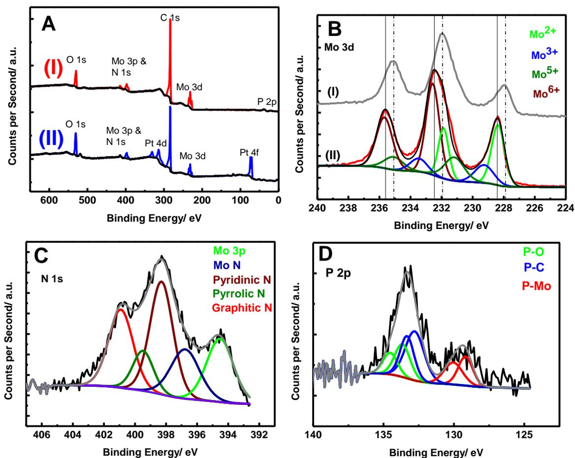
**Figure 4.** XPS survey spectra of DG-MoC (A-I) and Pt/DG-MoC (A-II) catalysts. B) XPS spectra of Mo 3d region of DG-MoC (II) and Pt/DG-MoC (I) catalysts. The inserted text colour matches the corresponding peak colour. Y axis presents different scales for each spectrum. C) Deconvoluted XPS spectrum of N 1s area of DG-MoC. D) XPS components of the deconvoluted P2p region of DG-MoC catalyst.
