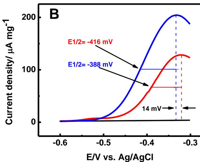
**Figure 5.** A) Cyclic voltammograms of 10% Pt/C (red line), Pt/DG-MoC (blue line), NG (green line in main figure and the insert) and DG-MoC (black dashed line in main figure and the insert) in  $N_2$  saturated
