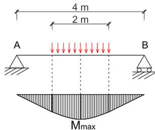
Figure 12. Arrangement of bending test with bending moment diagram (beam span  $L=4$  m).
