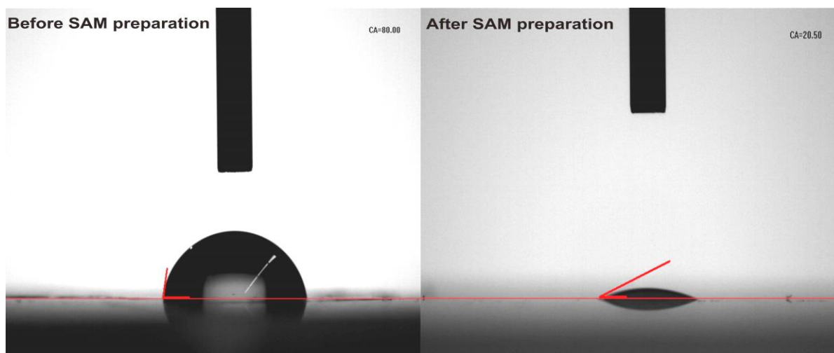
Figure 7: Contact angle of the delay line surface before and after the SAM preparation
