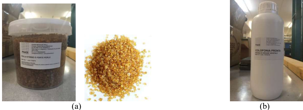
Figure 4. Natural resins used for repair: (a) Bone glue, (b) Rosin.
