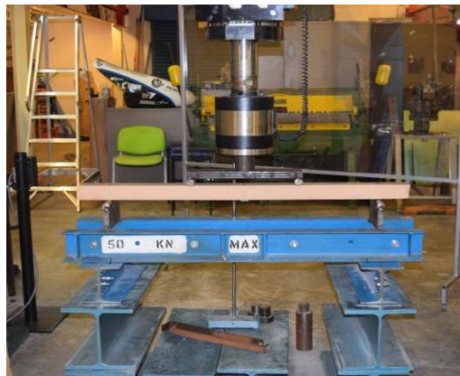
Figure 1. Test set-up (span between supports = 1004 mm and load span = 400 mm).
