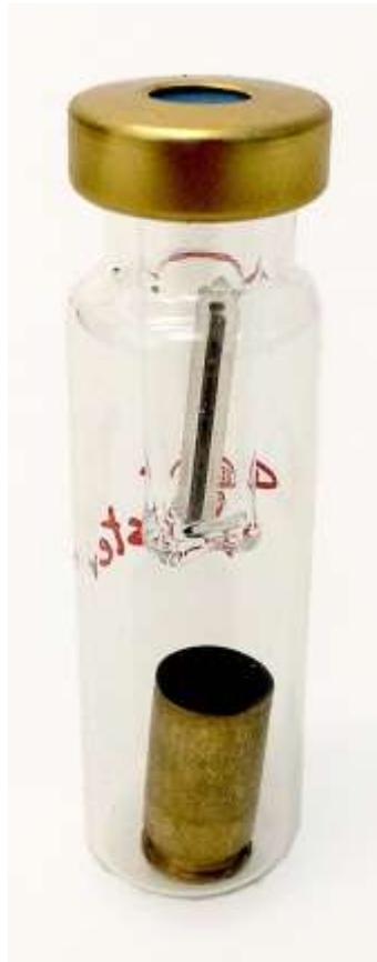
Figure 5 – Sampling of cartridges using HSSE, as suggested by Gallidabino et al. The HSSE extraction bar is put in a special insert in the extraction vial, just above the cartridge to analyse.
