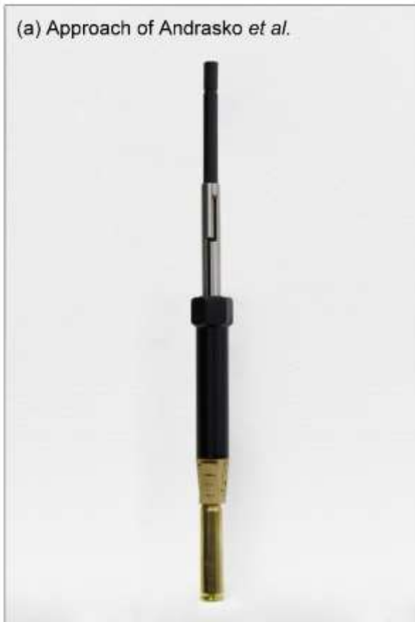
Figure 4 – Sampling of a 5.56 mm NATO spent casing using SPME, as suggested by (a) Andrasko et al. (using a cork to stop the opening) and (b) Wilson et al. (through putting the shell/cartridge in a vial).
