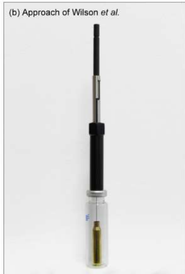
Figure 4 – Sampling of a 5.56 mm NATO spent casing using SPME, as suggested by (a) Andrasko et al. (using a cork to stop the opening) and (b) Wilson et al. (through putting the shell/cartridge in a vial).
