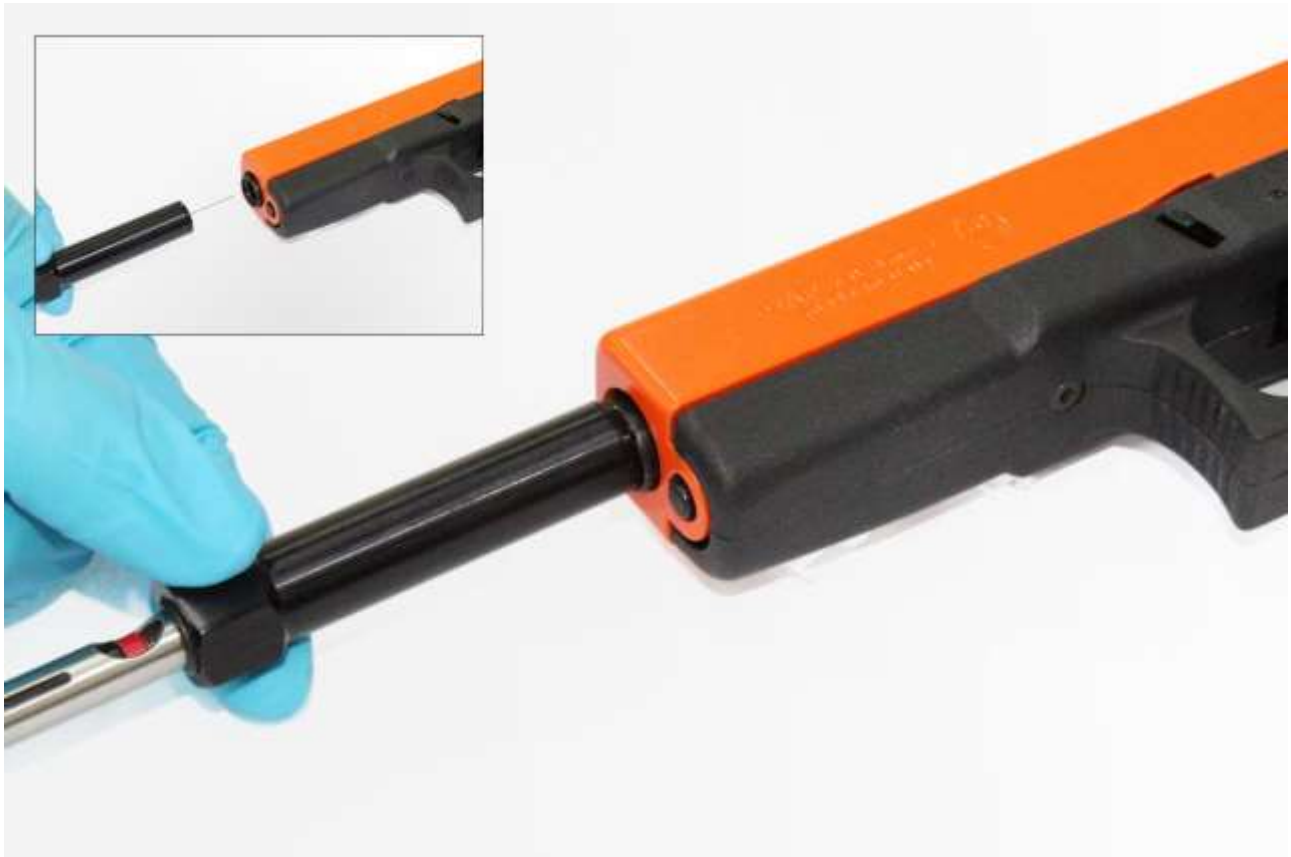
Figure 3 – Sampling of a 9 mm Parabellum pistol from the muzzle using SPME, as suggested by Andrasko et al.
