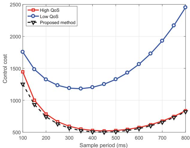
Fig. 3. Control cost versus control sample period.
