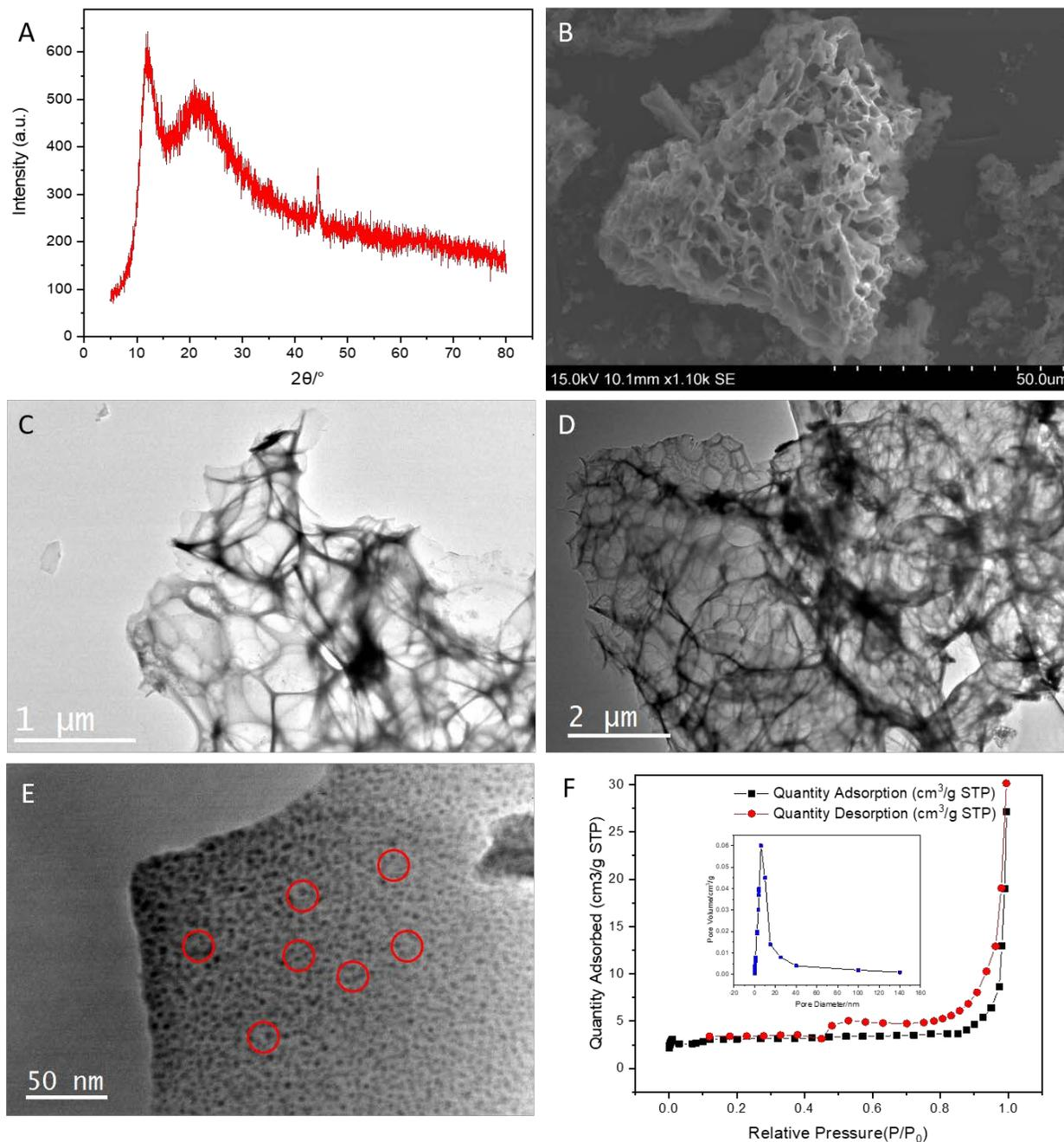
**Figure 1.** (a) XRD pattern and (b) SEM image of NiO/c-ESM, TEM image of (c) c-ESM and (d) NiO/c-ESM, (e) selected area TEM from (d), (f) BET analysis of NiO/c-ESM, inset: pore size distribution of NiO/c-ESM corresponding to (f).
