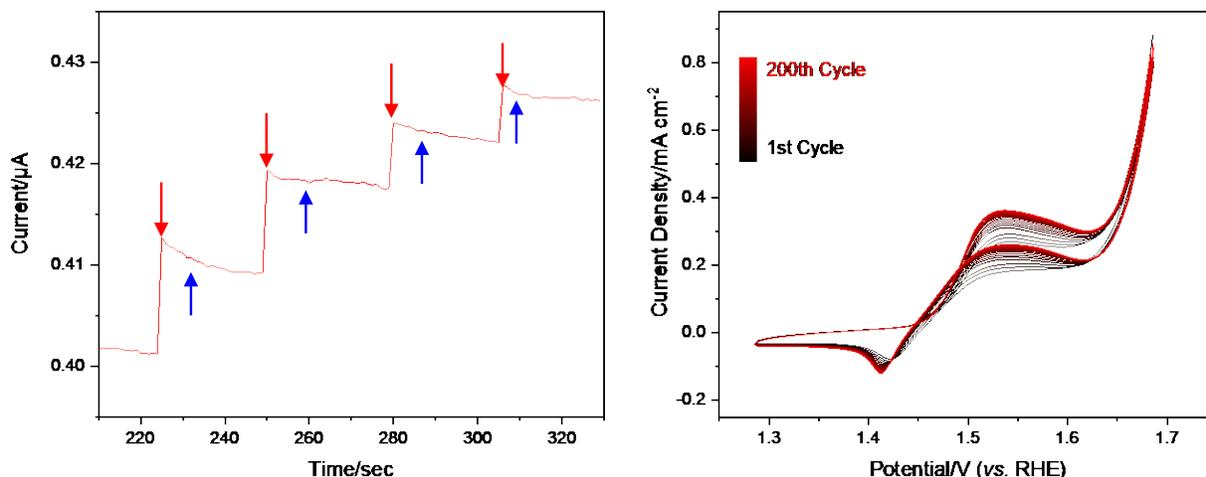
**Figure 6.** (a) The current responses to the addition of urea and different interfering species: 2.0 mM glucose, 2.0 mM Na<sup>+</sup>, 2.0 mM K<sup>+</sup>, 4.0 mM Cl<sup>-</sup> and 2.0 mM uric acid. (d) Cycling stability tests of NiO/*c*-ESM in 1.0 M KOH with 0.33 M urea at a scan rate of 50 mV s<sup>-1</sup>.
