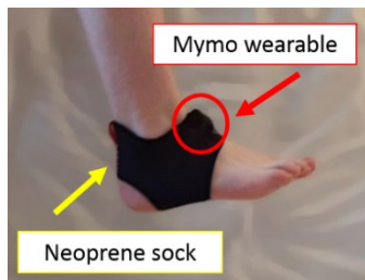
FIGURE 2. Attachment of the Mymo wearable with neoprene sock
