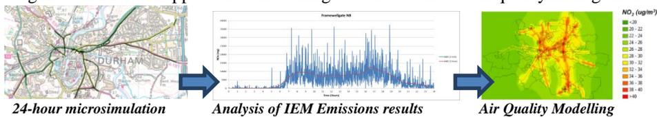
ADMS-Urban (CERC, 2006) was used for this research as it is user friendly, stable and has been extensively validated by over 70 UK local authorities (Riddle *et al.*, 2004). In this assessment modelled NO<sub>x</sub> values were converted to NO<sub>2</sub> using the DEFRA ‘NO<sub>x</sub> to NO<sub>2</sub>’ calculator (DEFRA, 2012).
