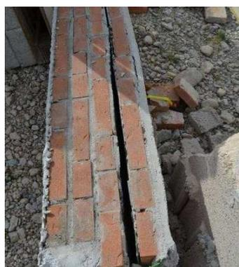
**Figure 25 – Detail of a brick masonry ring beam after failure**
