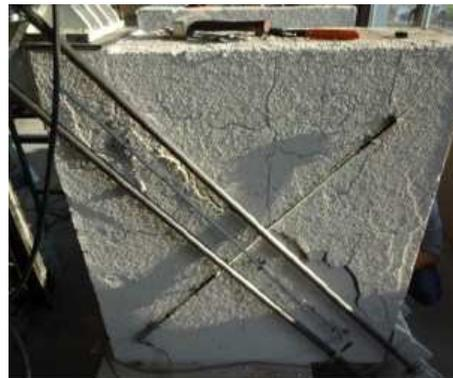
**Figure 9 – Failure mode for panel reinforced with mortar type RO**
