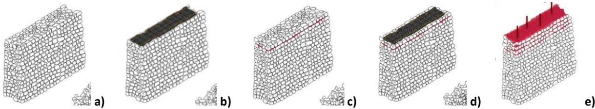
**Figure 19** – Construction methods of a reinforced masonry ring beam: a) removing the upper part of the existing wall; b) applying the first mortar layer reinforced with the GFRP grid; c) applying the stones; d) applying a second GFRP reinforced mortar layer; e) repeating the phases described in c) and d) until reaching the necessary height
