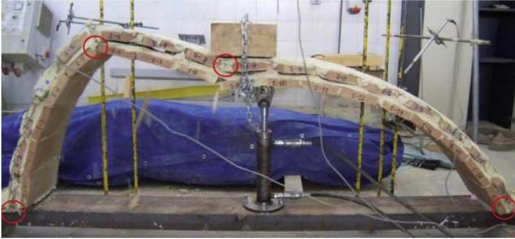
Figure 16 – Four-hinge mechanism
