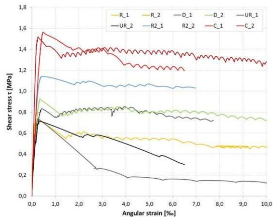
**Figure 11 – Shear stress vs. angular strain for unreinforced and reinforced specimens**
