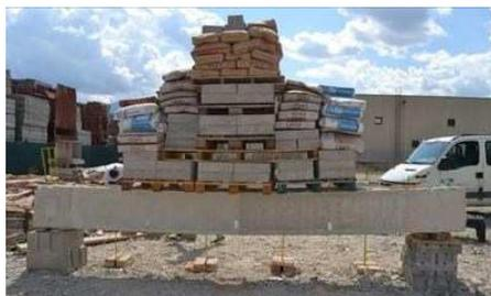
**Figure 22** – Bending test set-up
