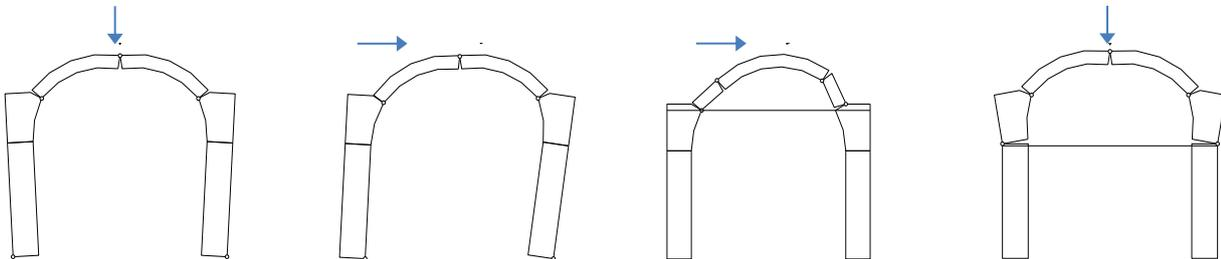
Figure 12 – Hinge mechanism for arch structures
