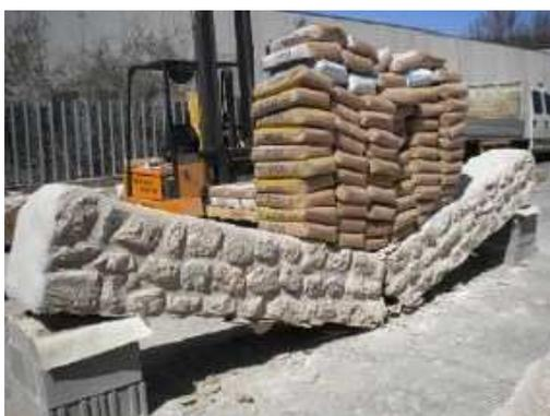
**Figure 24 – Failure of a stone masonry ring beam**
