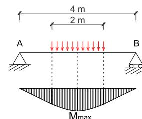
**Figure 23** – Test arrangement and bending moment diagram
