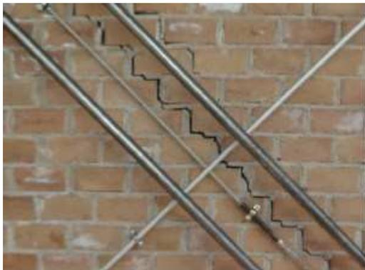
**Figure 8 – Failure mode for unreinforced panel**
