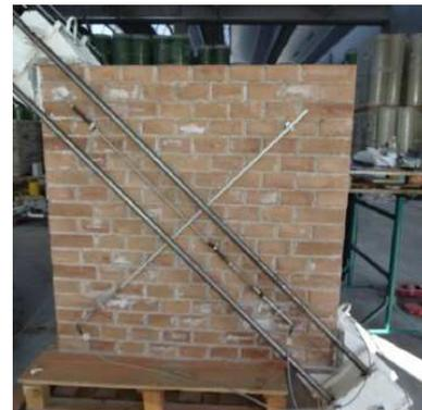
**Figure 7** – Arrangement of the instruments during the test
