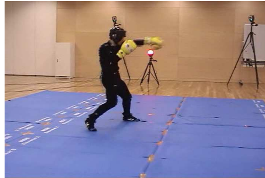
Figure 3: The shadow boxing motions of several boxers were captured using an optical motion capture system.
