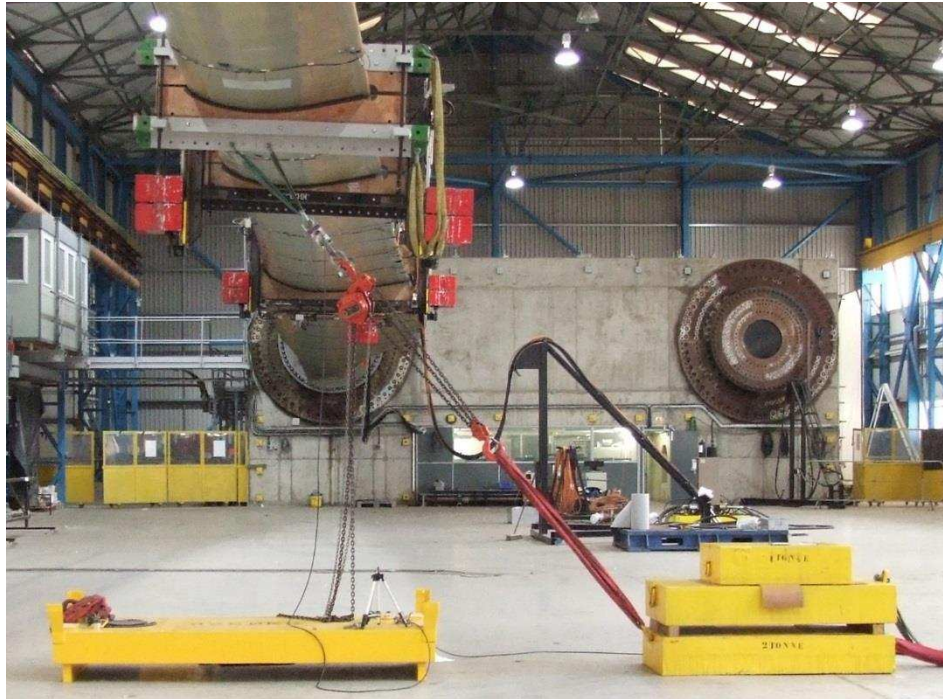
Figure 4. Combined load test configuration
