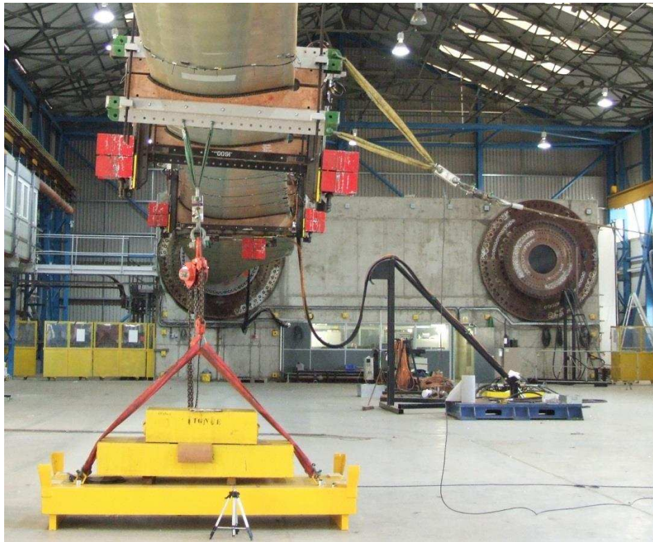
Figure 2. Flapwise calibration pull configuration also showing edge winch cable
