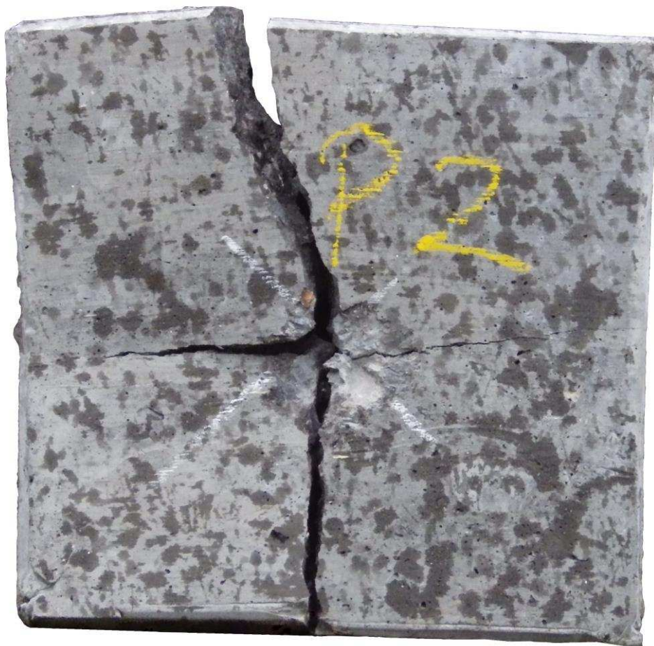
Figure 9 – Plain slab after one shot
