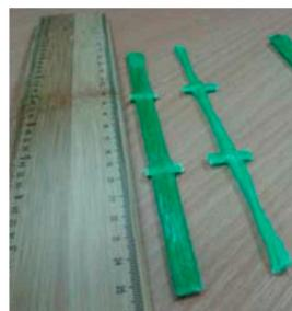
**Figure 6.** Specimens obtained from the  $66 \times 66$  mm<sup>2</sup> GFRP grid.
