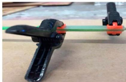
**Figure 7.** Detail of the epoxy tabs glued at both ends of the specimens.
