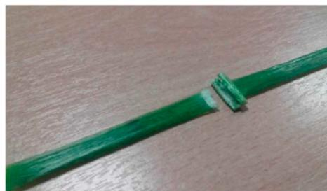
**Figure 10.** Partial fiber-failure at the GFRP grids joint.
