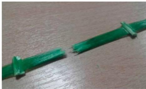
**Figure 9.** Catastrophic collapse of the GFRP sample.
