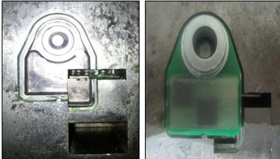
Figure 6 – First Moulding Pin Clamping Mechanism
